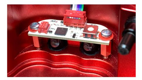
Optoelectronic TTL-Converter for OLYMPUS cameras for ISOTTA EM1-II and EM1-III underwater housings
