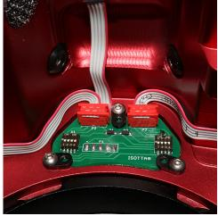
Optoelectronic TTL Converter for NIKON for ISOTTA housings of former years, including 2 pcs Optical Bulkheads with built-in LED
